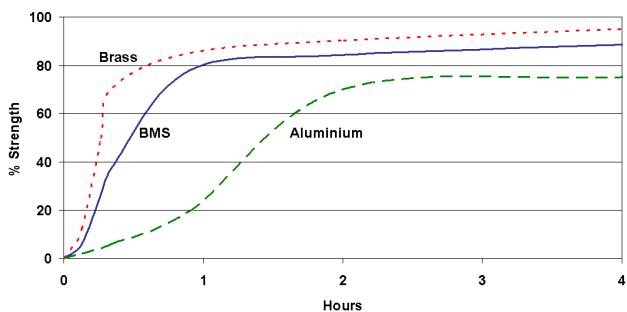
Cure times are typical at 23°C. Copper and its alloys will follow the faster cure while oxidised or passivated surfaces like stainless steel will tend towards the slower curve. Lower temperatures or large gaps will tend to extend the cure time. To reduce the cure time the use of Permabond A905, or heat, can be considered.
