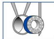
For larger components use thixotropic products to prevent run off. Take care to ensure adhesive does not enter ball races or other mechanisms.
